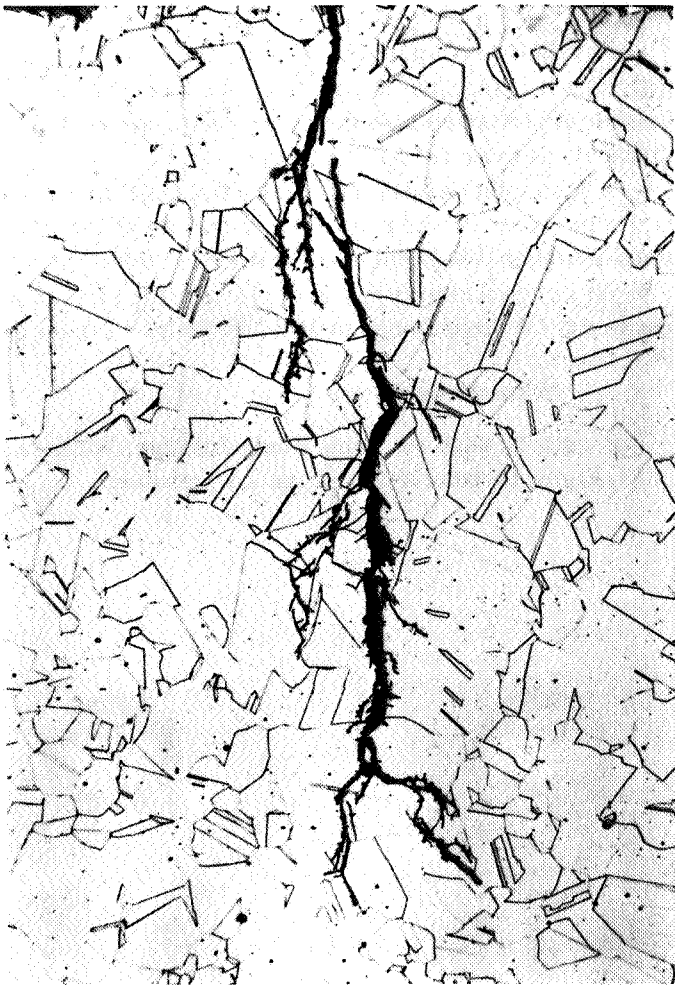
Figure 8. Micrograph of a small crack (Breda Institute).
